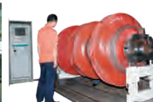
□ 三级双吸泵叶轮动平衡测试 Three impellers double-suction impeller dynamic balance test
